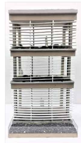
Detail physical detail model shows and tests practicality of details designed for green double skin facade.
